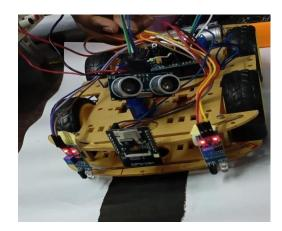
The control option is provided where the automatic can be switched to manual control by sliding control bar on the web user interface. When it is switchedon, the user will be able to control the robot using a web server that displays a live video streaming. The wireless communication is established between the user and the robot through internet, this is made possible with the help of ESP32 CAM Wi-Fi [4] module.
