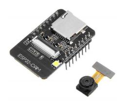
The ESP32-CAM AI-Thinker [8] is one of the most popular ESP32 development boards with camera – it comes with a lot of useful features and costs around **\$7 or less**! It features a ESP32-S chip and comes with a "regular" 2MP OV2640 [8] camera. This board has 4MB PSRAM, which is used for buffering images from the camera into video streaming or other tasks and allows you to use higher quality in your pictures without crashing the ESP32.
