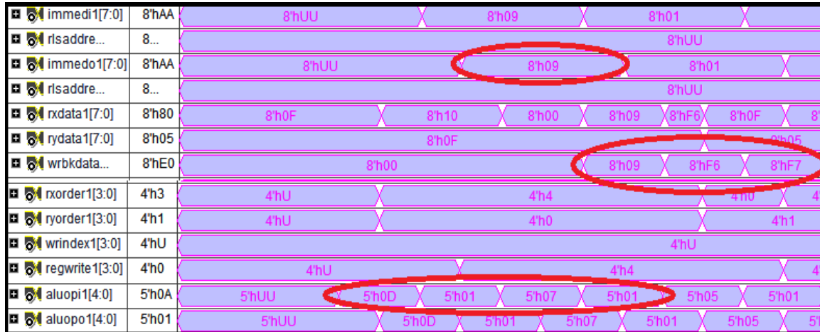
Figure. 3.5.c: showing the registers used, destination register address, data in registers and the opcode of instructions.
